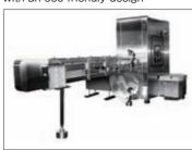
The lubricant has been changed from grease to oil in order to reduce the amount of lubricant used and lower the noise level.
