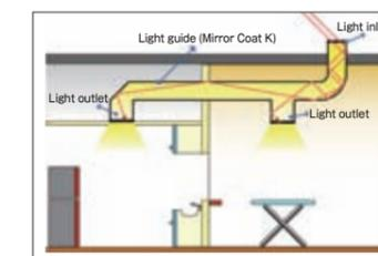
This is a system that uses a duct with a mirror finish-coated interior to reflect and direct natural light into places where a normal window cannot be installed. This system is expected to reduce CO<sub>2</sub> emissions by assisting energy conservation.
